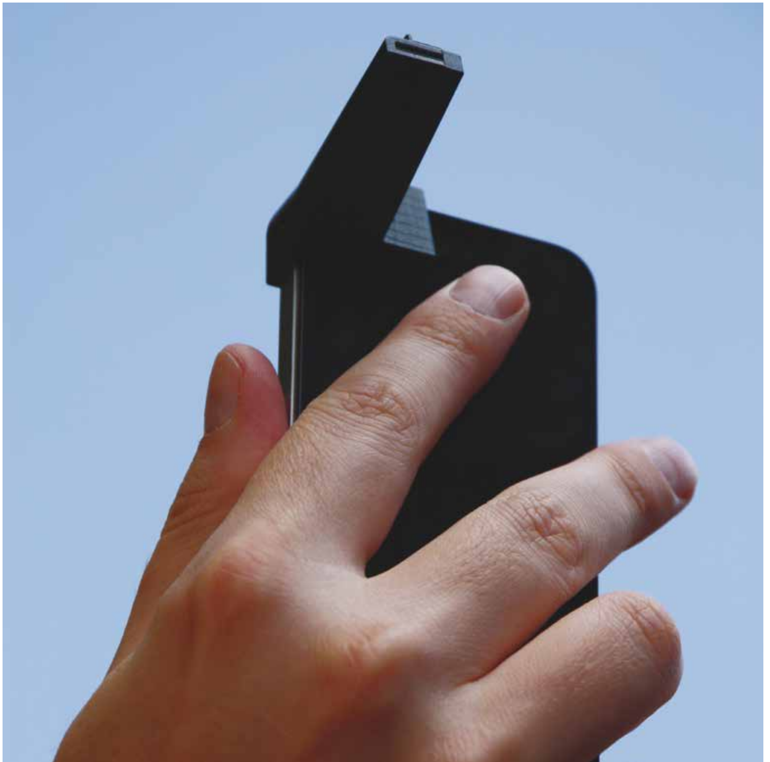
iSPEX, an add-on with complementary app, instantly turns a smartphone into a scientific instrument to measure dust in our atmosphere. Credit: iSPEX/Leiden Univ.
